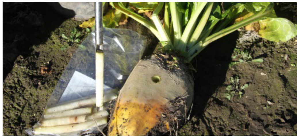
A beet corer samples the whole gradient of bulbs more accurately than chopping.
